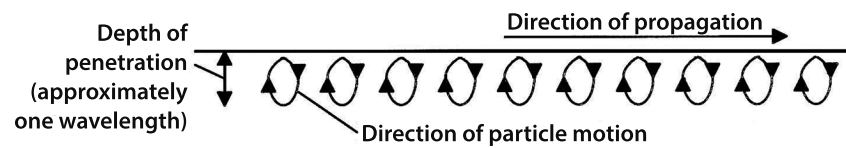
Figure 3.5 – Plate waves cause the thin plate to flex
